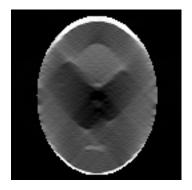
Example with 22 views uniformly spread along 90 degrees, without any noise. The constraints used are the data from measurements, and various a *priori* on : the pixel range( $x \in [0; 1]^N$ ), the total variation, and the support.
